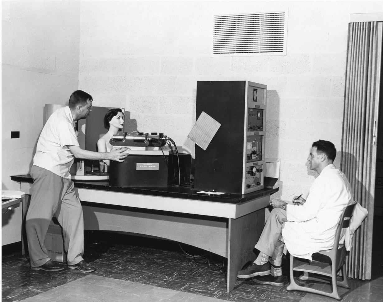
Marshall Brucer, far left, was the first chairman of the ORINS Medical Division, and was responsible for a highly successful radioiodine-uptake-calibration program - note the mannequin loaded with a known level of mock iodine was used to calibrate instrumentation (Photo courtesy of Oak Ridge Associated Universities)
